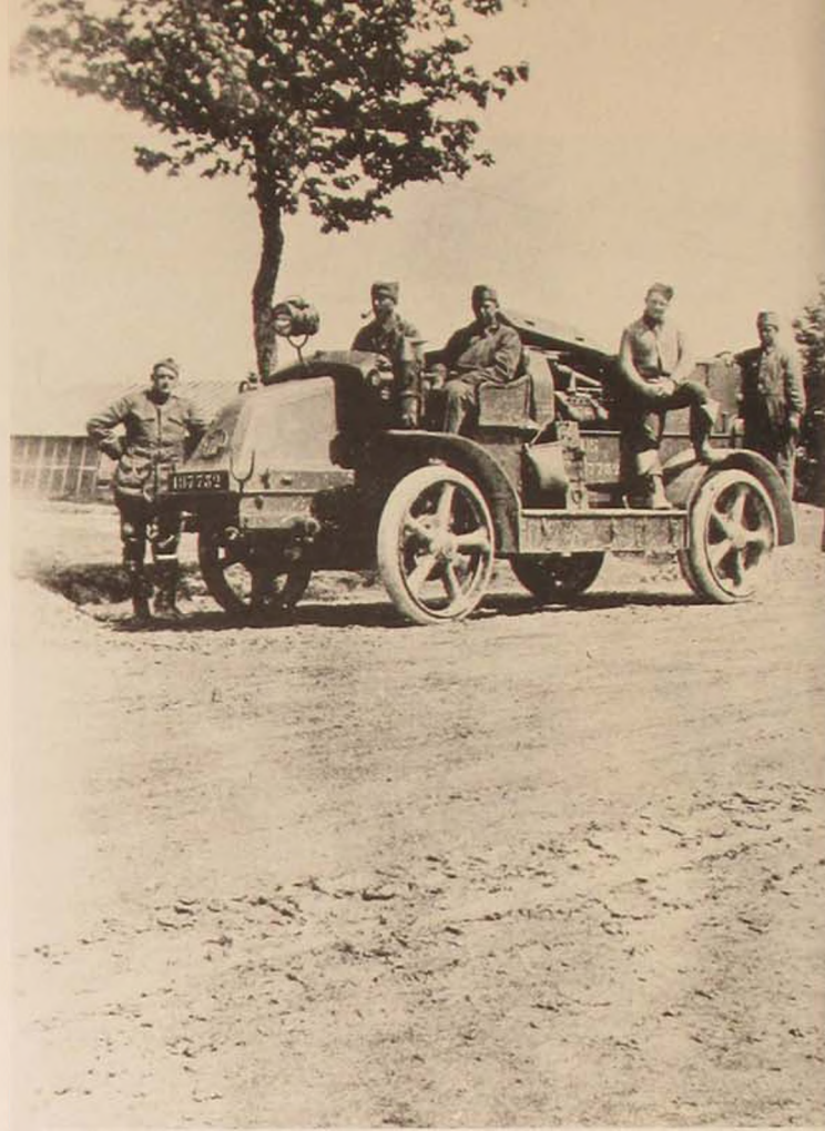
A fully inflated Caquot balloon (above) with one passenger aboard floats on the air above its handling crew and winch trucks. . . . The winch truck (right) used by U.S. forces during World War I could lower a balloon as fast as 1600 feet per minute. It could also tow an inflated balloon at a speed of five miles per hour, even faster in an emergency.
