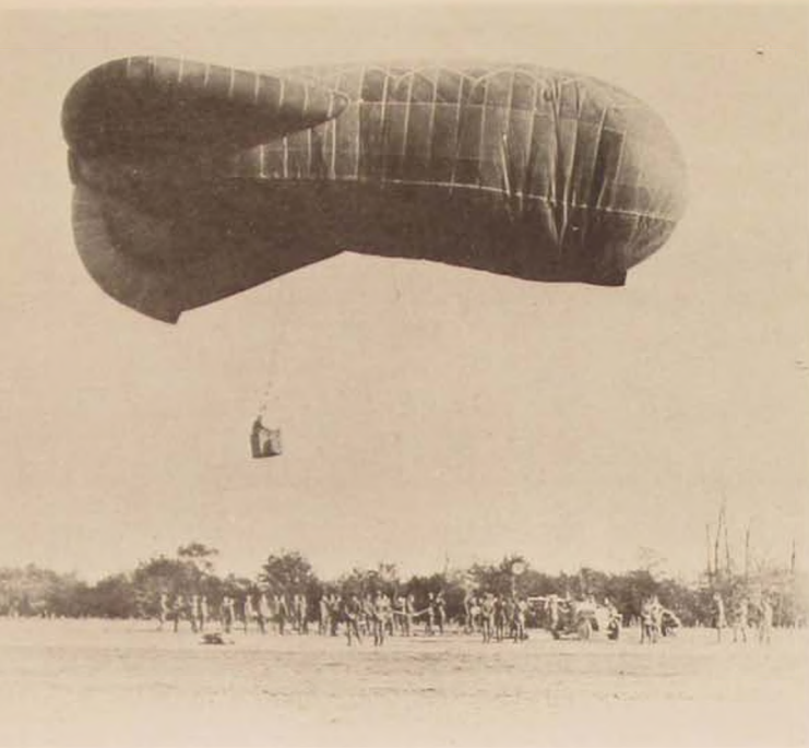
A fully inflated Caquot balloon (above) with one passenger aboard floats on the air above its handling crew and winch trucks. . . . The winch truck (right) used by U.S. forces during World War I could lower a balloon as fast as 1600 feet per minute. It could also tow an inflated balloon at a speed of five miles per hour, even faster in an emergency.
